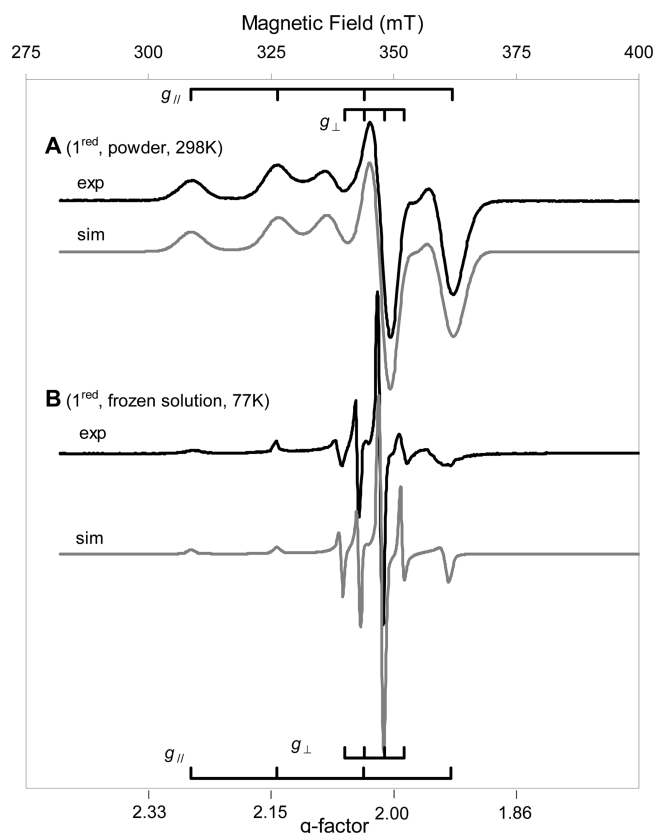
Figure 5. X-band (9.65 GHz) EPR spectra of 1 red . (A) Powder spectrum at room temperature (298 K); experimental (exp, dark line) and simulation (sim, gray line). (B) Frozen DMF solution (0.15 M of 1 red ) spectrum at 77 K; experimental (exp, dark line) and simulation (sim, gray line). Spectra were acquired as described in the Experimental Section, and the other conditions were as follows: modulation frequency, 100 kHz; modulation amplitude, 0.2 mT; microwave power, 635 \mu\text{W} . Spectra were simulated as indicated in the Experimental Section, with the parameters summarized in Table 2.
